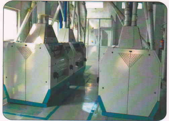
Latest Corn De-Germinator flexible operation Flaking grits - Wet Hulling Snack grits - Dry Hulling
